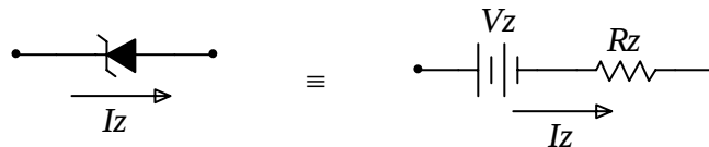
Figure 2. Zener diode model in the breakdown region
